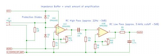
Figure 3.4: Schematic of the amplification circuitry used.
