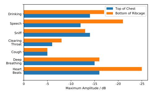
Figure 4.2: The maximum amplitude in the audio for different events of interest for the two placements evaluated (3 and 4 in fig. 4.1).
