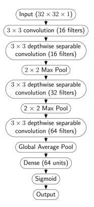
Figure 6.3: Architecture used for asthma detection on-device
