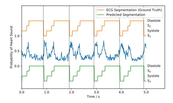
Figure 5.4: Predicted segmentation by the proposed algorithm compared to the ECG ground truth, when user is at rest. The emission probability used by the HSMM are also marked.
