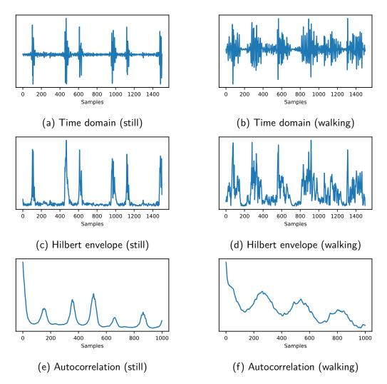
Figure 5.1: Visualisation of the stages in algorithm 1, for both still and walking situations. Audio sampled at 500Hz.
