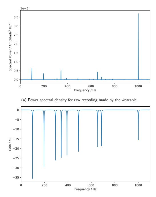
(b) Frequency response of filter applied to raw recordings.
