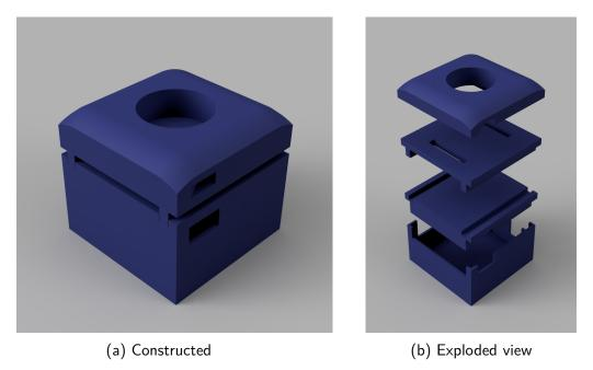
Figure 3.5: Renders of the final casing used for the wearable.
