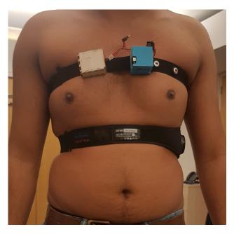
Figure 4.3: Photo of the author wearing the microphone and ground truth devices.
